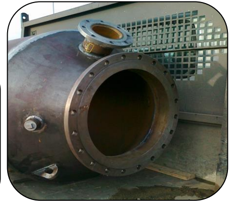
De-sulphurisation unit operating at 75°C rebuilt using 201 Ceramic Repair Paste and resurfaced using 205 Ceramic HT Fluid
