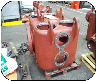
Sea water filter operating at 95°C coated with 205 Ceramic HT Fluid
