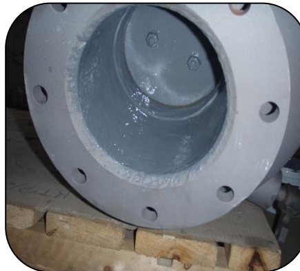
De-sulphurisation unit operating at 75°C rebuilt using 201 Ceramic Repair Paste and resurfaced using 205 Ceramic HT Fluid
