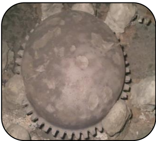
Ammonia Liquor process vessel operating at 100°C resurfaced with 205 Ceramic HT Fluid
