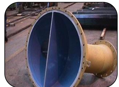
Process pipework abrasive blast cleaned and coated with 203 Super Flow
