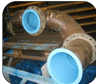
Process pipework abrasive blast cleaned and coated with 203 Super Flow
