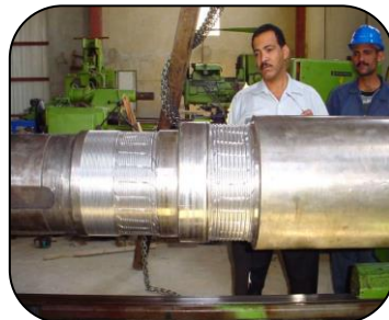
Quarry crusher shaft rebuilt using 107 Metal repair Paste XL (India)
