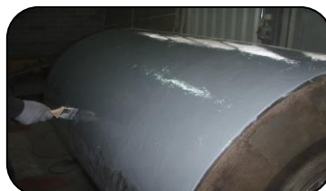
Belt rollers resurfaced using 102 Metal Repair Fluid and Aluminium Oxide
