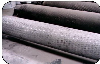
Belt rollers resurfaced using 102 Metal Repair Fluid and Aluminium Oxide
