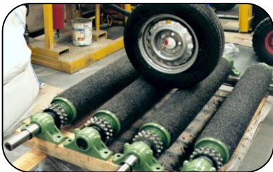
Resurfacing of brake test rollers using 102 Metal Repair Fluid
