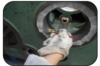
Metal surfaces rebuilt and machined using 101 Metal Repair Paste
