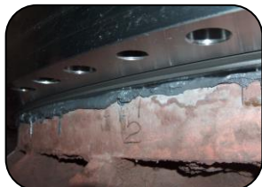
Gasket chocking using 101 Metal Repair Paste
