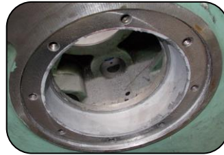
Metal surfaces rebuilt and machined using 101 Metal Repair Paste
